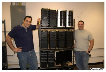
We have constructued and managed a 19-node GPU-enabled cluster named Jarvis for systems courses including CS546, CS550, CS451, CS554, et
